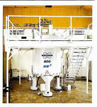
AVANCE 800 US<sup>2</sup> complete NMR system in operation at Bruker's application laboratory
