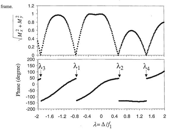
Fig. 1. The excitation profile by the composite pulse  $90_x^\circ 90_y^\circ 90_{-x}^\circ 90_{-y}^\circ$  (top) and the corresponding phase (bottom). A phase inversion, denoted by  $\lambda_1$  to  $\lambda_4$ , occurs at each null.
