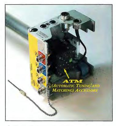
A This new TXI Probe from Bruker incorporates an AUTOMATIC TUNING AND MATCHING (ATM) ACCESSORY into the probe base. ATM allows the spectrometer to perform tuning and matching under computer control, letting you and your colleagues concentrate on analysing results, not monitoring acquisition of spectra.
