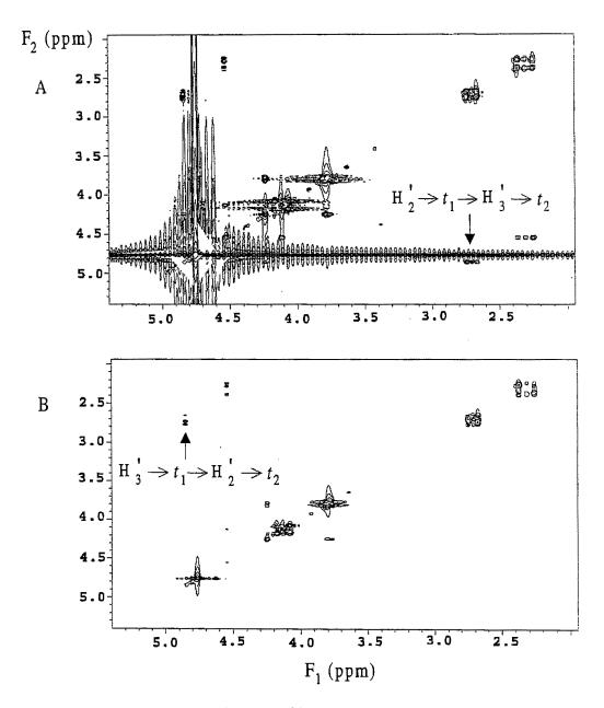
Fig. 2. Constant-time  $^1H$  -  $^1H$  ( $^{31}P$ ) COSY spectra of 4.0 mg of d(GC) in 600 ml D<sub>2</sub>O recorded on a Varian Unity Plus 600 MHz instrument without (A) and with (B) WATERGATE.
