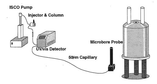
In summary, we expect to put this probe to great use in cases where we are extremely sample limited, or where the sample contains several compounds. We will be able to do more interesting experiments to each compound by using stop-flow chromatography. And finally, by using mobile phase gradients, we will be able to improve the chromatography and concentrate the longer-retained compounds.
