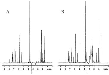
**Figure 2**. 1D spectra of a 750 uM sample, as in Figure 1, (A) in DMSO-D6 and (B) in DMSO-H6. The solvent peaks were suppressed with a WET sequence. The number of scans was set to 128.
