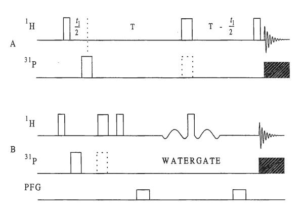
Fig. 1. Constant-time  $^{1}\text{H}$  -  $^{1}\text{H}$  ( $^{31}\text{P}$ ) COSY pulse sequence for measuring  $J_{\text{H-P}}$  coupling constants without (A) and with (B) WATERGATE.
