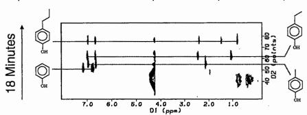
mixture of four phenols. The injected volume contained only 2 micrograms of each compound. Horizontal slices through the data show NMR spectra of the individual components. Thus we were able to demonstrate both our ability to detect small amounts of material, and our ability to separate a mixture using chromatography.
