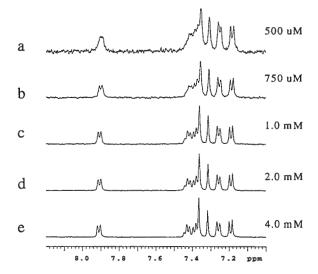
Figure 1. The aromatic region of a compound of molecular weight 600 with different concentrations, as labeled in the figure. The number of scans was set to 128.
