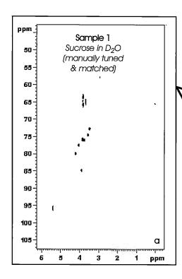
$^1H^{-13}C$  HSQC spectra of two Sucrose in  $D_2O$  samples that differ in ionic strength taken with a TXI Probe. Sample 1 was manually tuned and matched. After changing to Sample 2, spectra were obtained (b) without tuning or matching and (c) with Automatic Tuning and Matching Accessory enabled. ATMA enables autosampling with sensitive inverse probes at high field, ideal for fully automated biological NMR screening techniques.
