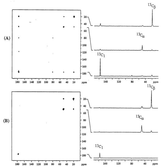
Figure. Phase sensitive 2D <sup>13</sup>C CPMAS homonuclear correlation spectra of triply labeled <sup>13</sup>C alanine recorded on a Bruker DMX 300. The sample spinning speed was adjusted to 7.2 kHz to avoid rotational resonance. The rotor-synchronized 180° pulses<sup>2</sup> (A) and the SFAM irradiation (B) were applied during the 20.8 ms mixing time. The slices in the right are the phase-sensitive cross sections showing relative intensities of the cross peaks.
