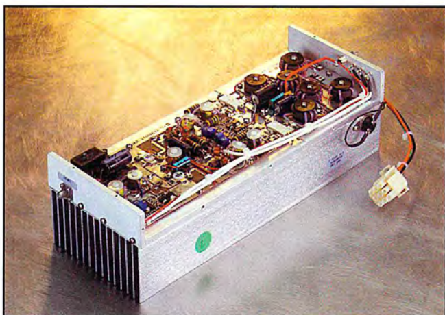
6 MHz to 220 MHz, 300 W, NMR Module
