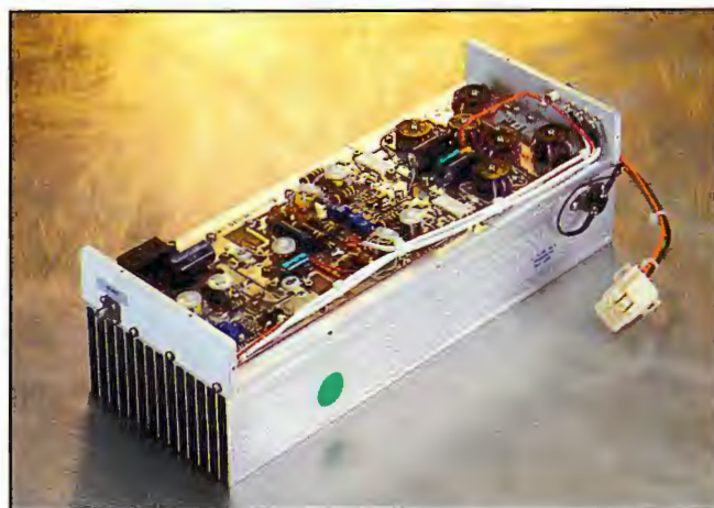
185 MHz to 500 MHz, 125 W, NMR Module
