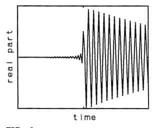
FIG. 1. The beginning of a simulated FID comprising six sinusoids with amplitude ratio 20000:1:2:4:2:1 and equal damping factors. This signal was filtered by a multistage digital decimation FIR filter and an oversampling ratio of 256:1.
