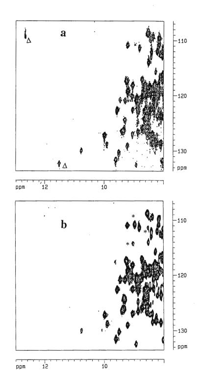
Figure 1. a)  $^{1}H^{-15}N$  HMQC spectrum of stromelysin-inhibitor complex using presaturation for water suppression. b)  $^{1}H^{-15}N$  HMQC spectrum of stromelysin-inhibitor complex with Spin-Echo water suppression. The excitation center was 3.2 ppm from the water peak.
