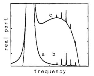
FIG. 2. a) Theoretical spectrum of the simulated signal. b) DFT of the recorded digital FIR filtered signal. c) DFT of the same signal with improper omission of the initial part in  $-t_s \le t < 0$ .
