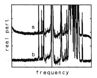
FIG. 3. Experimental 500 MHz spectrum of melezitose dihydrate obtained with a Bruker DMX 500. a) DFT with improper omission of the initial part  $-t_s < t < 0$  of the FID. b) DFT with inclusion of the initial part of the FID.
