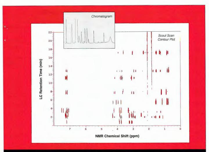
On-flow 500 MHz 'H LC-NMR data of a peptide mixture using Scout Scan and WET solvent suppression during an LC gradient. The sample was a 100  $\mu$ l injection of ~1 mg/mL peptides separated using a CH<sub>3</sub>CN:D<sub>2</sub>O solvent gradient (5% CH<sub>3</sub>CN to 50% in 22 min).
