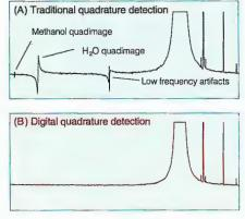
Bruker standard dynamic range sample, obtained with (B) and without (A) DQD
