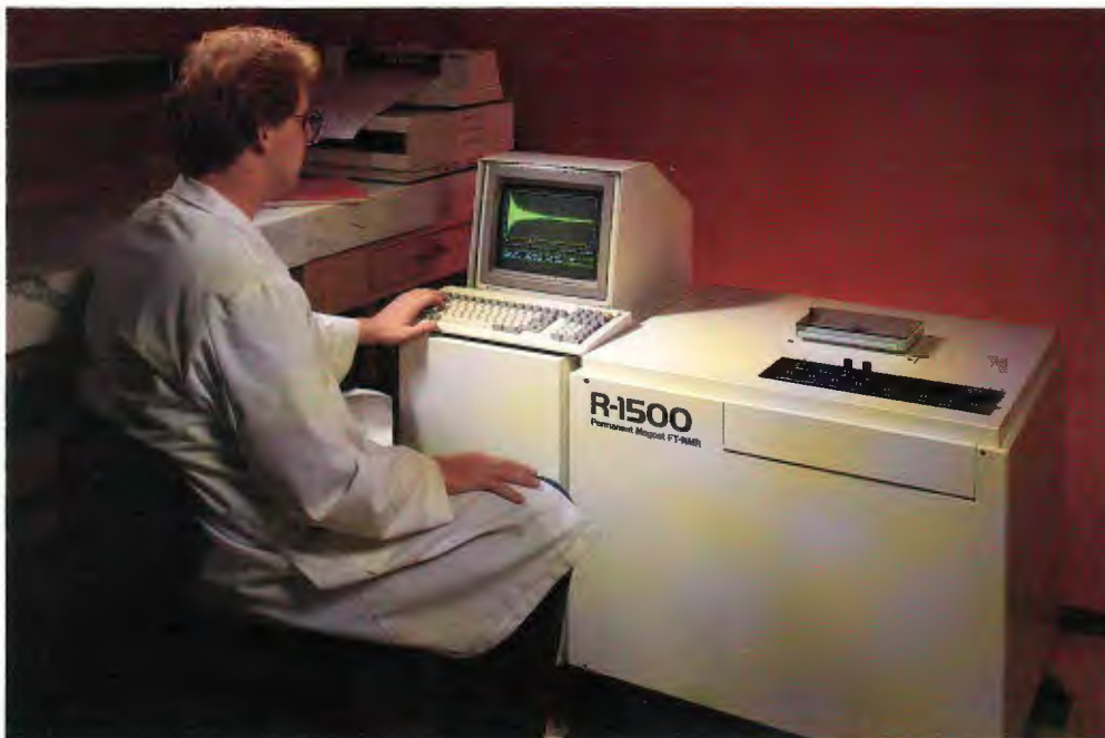
The Model R-1500 60 MHz Fourier Transform NMR Spectrometer. (Photo provided through the generous courtesy of the Department of Chemistry Teaching Laboratory, University of Massachusetts, Amherst, MA.)
