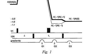
Pulse Sequence and the coherence pathway diagram for a 15N GE-HMQC experiment.
