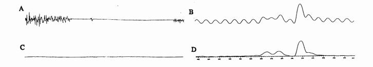
Figure 1. A comparison of (A) the corrupt fid 69 and (B) an f3 trace through the first F1F3 (<sup>1</sup>H-<sup>13</sup>C) plane of an HNCO experiment containing the corrupt fid, versus (C) the reacquired fid 69 and (D) the same f3 trace as (B) with the corrupt fid replaced in the data set (see below).
