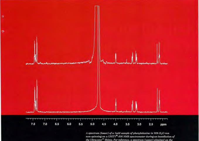
the Ultra•nmr<sup>™</sup> Shims. For reference, a spectrum (upper) obtained on the identical instrument equipped with enhanced shims.
