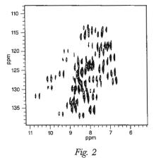
A 2P Ge-HMQC spectrum of 15N enriched BPTI. The sample was 2.6mM in 90% H2). The data collection time was 2.6 hours.
