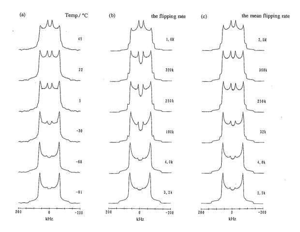
Figure 1. Temperature dependence quadrupole echo spectra of the deuterated phenyl ring of poly(Lphenylalanine): (a), observed spectra; (b), calculated spectra with one flipping rate; (c), calculated spectra with the normal distribution for the flipping rate.
