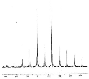
Figure 1. Ti spectrum of SrTiO, obtained at 28.17 MHz (4000 Hz spinning).
