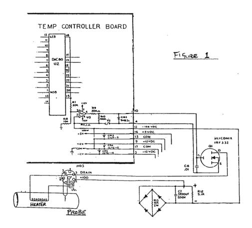
Referring to Figure 1: As designed, (at least on older Temperature Controllers, like ours) if the control circuitry U2, U3, etc. on the temp. controller board malfunctions and the gate (G) is driven high on the power FET (Q1), a thermal runaway will exist until fuse F2 blows, breaking the
