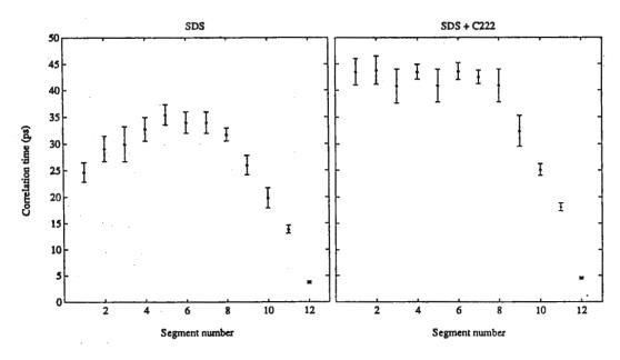
Fig. 2 Correlation time  $au_c^{ch}$  for the local motion of individual methylene segments.
