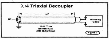
birdcage. The signal cable is connected in series with two balanced 110 pF capacitors to the matching loop (Fig 3). The pocket is located exterior to one loop of the birdcage, that is between two rungs, and matching adjustment is made by moving the paddle axially to vary the overlap of the matching loop with the birdcage loop. The matching range of the coil is sufficient to match empty or with a
