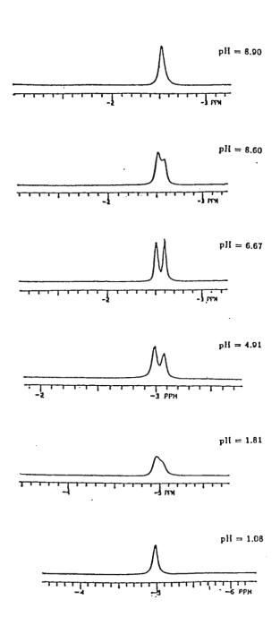
Figure 1. Proton decoupled <sup>31</sup>P NMR Spectrum of Phosphocreatine in mixture of D<sub>2</sub>O and H<sub>2</sub>O showing splitting as a function of pH at a temperature of 4.0°C.
