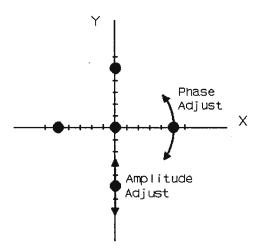
We have found this technique to be particularly robust due to its ease of application for both conventional quadrature RF adjustments, as well as its application to nonconventional amplitude and phase angle (45°, 60°, etc.) adjustments. Perhaps in this last application, this technique will have its greatest utility.
