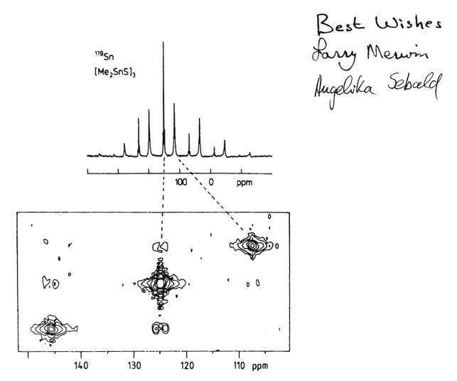
Figure 1: Conventional 119Sn CP MAS spectrum of (Me<sub>2</sub>SnS)<sub>3</sub> (top), together with an expansion (centre band region) of the <sup>119</sup>Sn CP-COSY contour plot.
