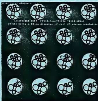
Fig. 2 —16 contiguous 1 mm slices FOV 6.4 mm, NEX 4. TR 150 msec, Field Strength 2T, TE 14 msec
