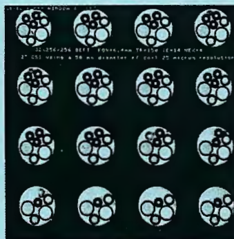
Fig. 2—16 contiguous 1 mm slices FOV 6.4 mm, NEX 4. TR 150 msec, Field Strength 2T, TE 14 msec
