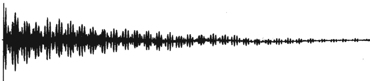
Fig.1. FID of polypropylene in 1,2,4 trichlorobenzene after 16 hours
