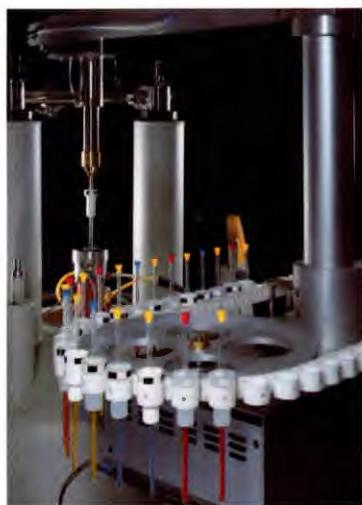
Full automation in NMR sample handling.
