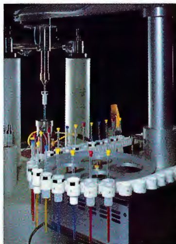
Full automation in NMR sample handling.
