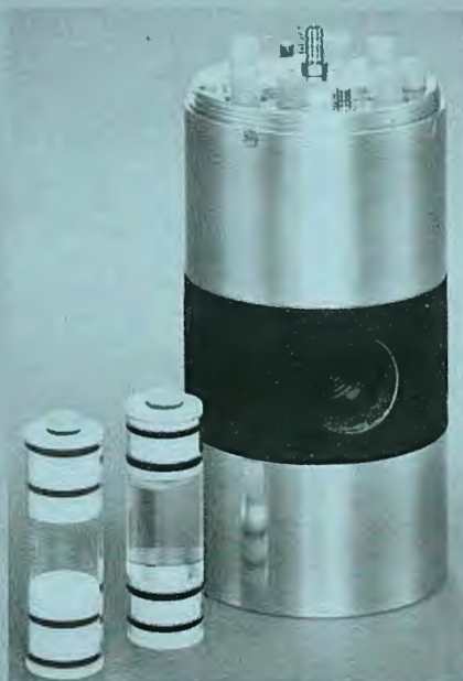
New solenoidal sideways-spinning probes provide enhanced sensitivity.
