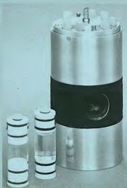
New solenoidal sideways-spinning probes provide enhanced sensitivity.
