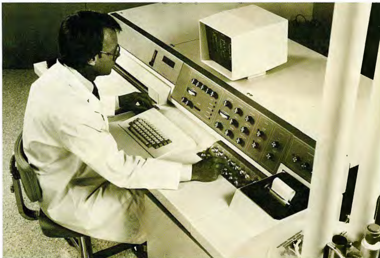
Varian XL-200 Superconducting FT NMR Spectrometer.
