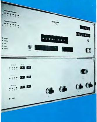
The ASPECT 2000 is a complete data acquisition and processing system which can be used efficiently wherever the time dependence of physical observables must be stored and analyzed. It is a high performance minicomputer with dual-input A/D converters and numerous interfaces. Together with its comprehensive software, the ASPECT 2000 offers unmatched capabilities for data-collection, calculation, analysis and output.
