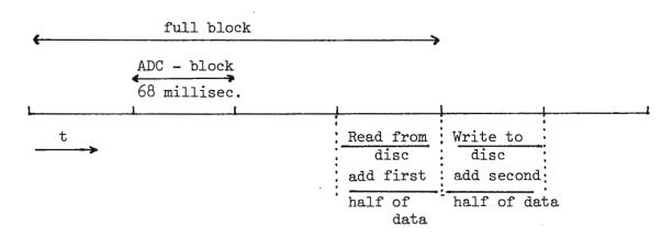
fig. 1 The basic principle of the data-acquisition and -reduction.
