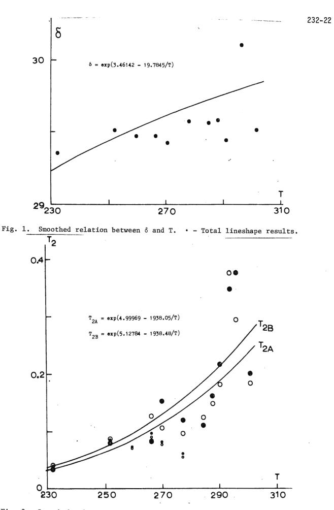
Fig. 2. Smoothed relations between  $T_{2A}$ ,  $T_{2B}$  and T. 0 -  $T_{2A}$  and • -  $T_{2B}$ Total lineshape results: smaller circles obtained from linewidth measurements
