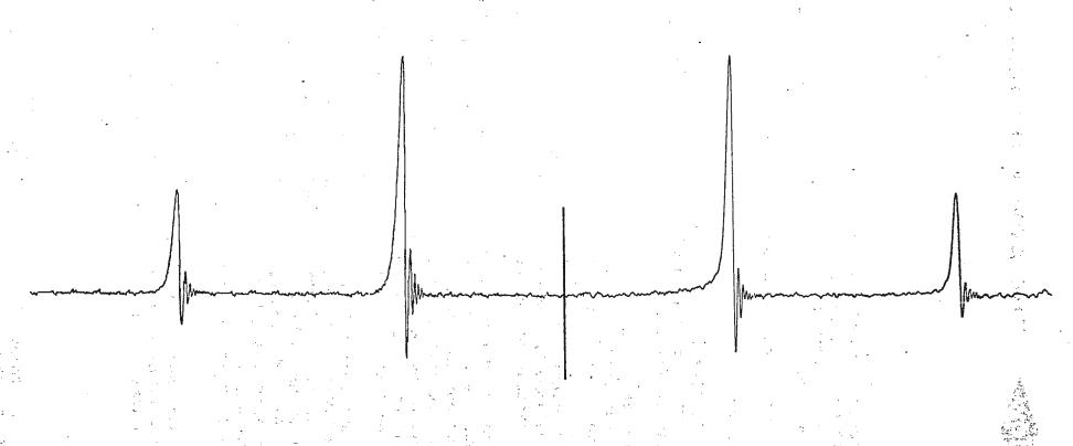
Continuous wave spectra of an AB system of spin-1/2 nuclei. One-half of the spectra is experimental; and one-half is a simulation, including simulated noise.
