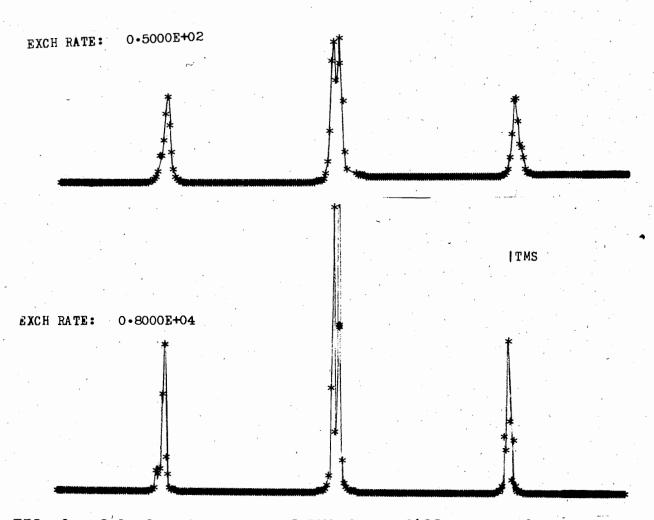
FIG. 2. Calculated spectra of DMA-d<sub>3</sub> at different exchange rates. Chemical shifts are -301.16, -313.96 hz;  $B_{11} = B_{22} = 151.86$  kg,  $B_{12} = 3.35$  hz.
