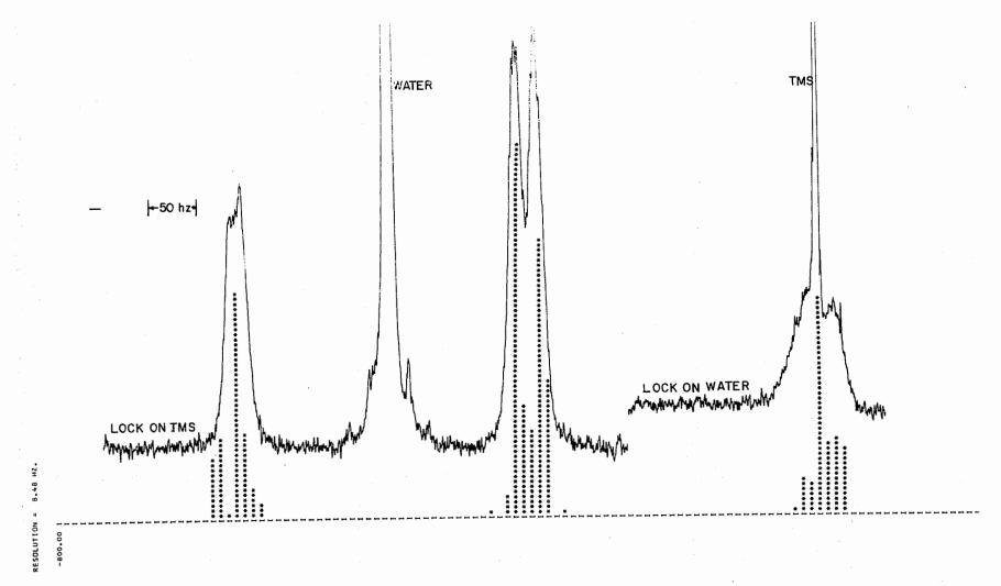
FIGURE 3. Observed and calculated NMR spectra of DMA-d $_3$  in a lyotropic nematic solvent at 25°c. Assigned parameters are shown with Figure 2. Spectrum taken at 100 MHz on a Varian HA-100.
