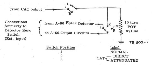
The leads were removed from the Detector Zero control-operated external input switch. This permits the use of a 10-turn pot in the Detector Zero control (for the benefit of those of us without the lock-pickers touch). The switch and pot were mounted in a convenient place on the A-60 front panel.
