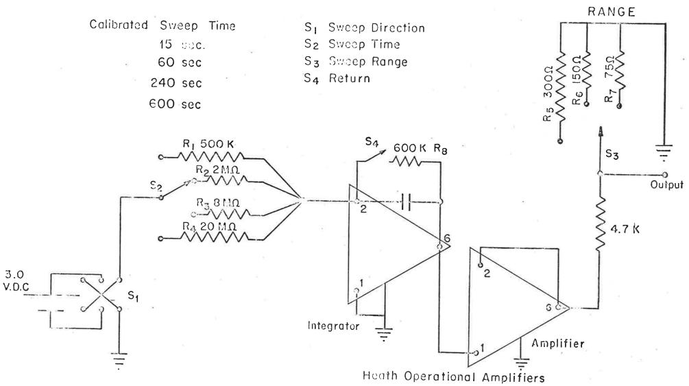
Resistors all ½ Watt Capacitor, 1mfd, 600 V.D.C. Frequency Sweep Unit
