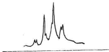
H^1 Resonance at 40 Mc/s of -OH_2- group in diethylamine.
