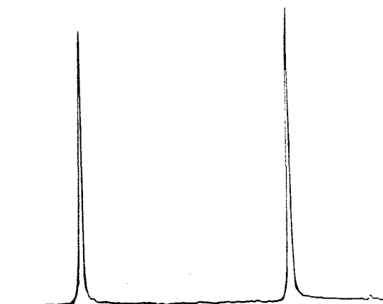
Figure 7: CP/MAS spectrum of 1.10g of HMB, taken with 12 scans. 5ms contact time, 1s delay time, 21 Hz line broadening. Spectrum at 25.12 MHz on a Bruker CXP-100.
