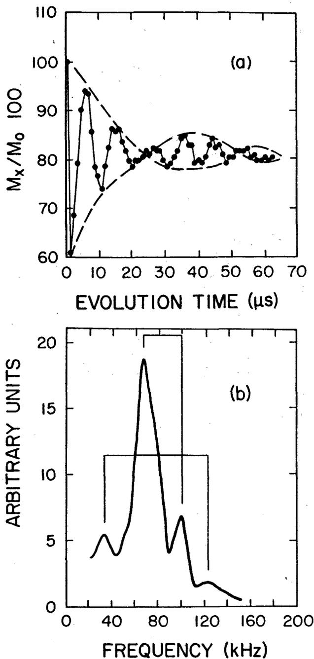
Figure 2: (a). Non-equilibrium proton spin magnetization ratio  $M_x/M_0$  as a function of the duration of the locking pulse for the  $\text{PdH}_x$  sample with  $X = 0.80$ . The amplitude of the locking pulse was  $8.40 \pm 0.40$  gauss. The dashed line is a guide to the eye to indicate the modulation. (b). Fourier transform of the transient data. Dominant and secondary doublets centered at about 80 kHz indicate tunneling splittings.
