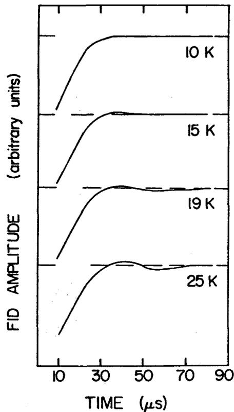
Figure 7: Examples of the proton free induction decay signal obtained from the  $\text{PdH}_x$  sample with  $X = 0.75$  in the temperature range 10 to 30 K.
