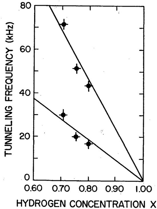
Figure 3: Concentration dependence of the two lowest tunneling frequencies in  $\beta$ -phase  $\text{PdH}_x$ . The straight lines are guides to the eye; they indicate a  $(1 - X)$  dependence.
