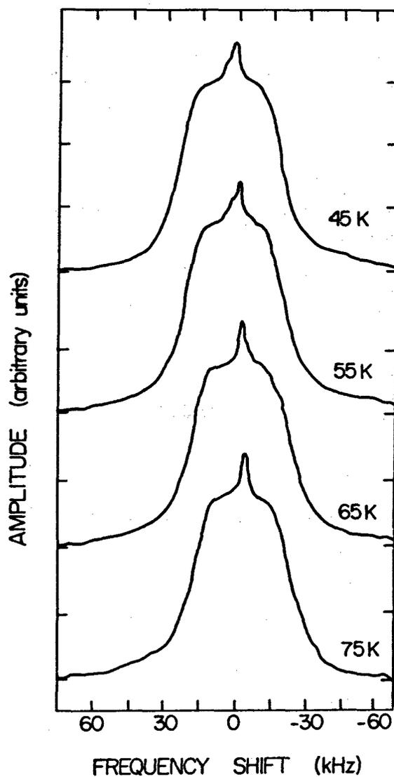
Figure 5: Examples of the proton spin absorption lineshape measured for the  $\text{PdH}_x$  sample with  $X = 0.71$  in the temperature range 30 to 80 K. The width of the central feature at half height is about 7 kHz.
