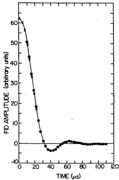
Figure 4: The proton free induction decay signal for the  $\text{PdH}_x$  sample with  $X = 0.75$ . The dots are experimental data and the full curve the fit to the empirical function given by equation (3). The crosses are data points obtained using a magic echo sequence.
