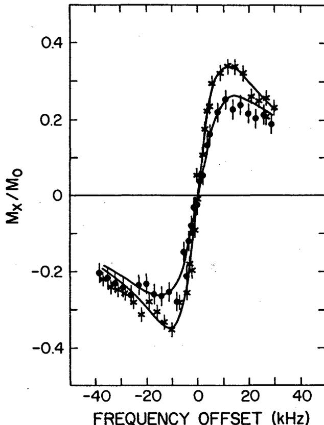
Figure 1: The proton spin magnetization ratio  $M_x/M_0$  as a function of frequency offset for the  $\text{PdH}_x$  sample with  $X = 0.75$  for spin temperature experiments using a 50 msec rf pulse (crosses) and a 3 sec rf pulse (dots) and with  $H_1 = 7.6 \pm 0.4$  kHz. The solid lines are the theoretical fits to equations (1) and (2).
