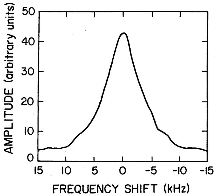
Figure 6: Proton spin absorption spectrum deduced from the Hahn echo for the  $\text{PdH}_x$  sample with  $X = 0.71$  at 40 K. The spectral width at half height is 7.2 kHz.
