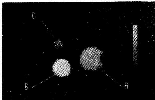
Fig. 2. Test object imaging. Cylindrical sample of 7 cm diameter filled with water in which three tubes A, B, C, with 1 mM Fremy's salt in phosphate buffered saline are set. Oxygen partial pressure A : 170 mmHg, B : 94 mmHg and C : 270 mmHg. (EPR irradiation 10 W).
