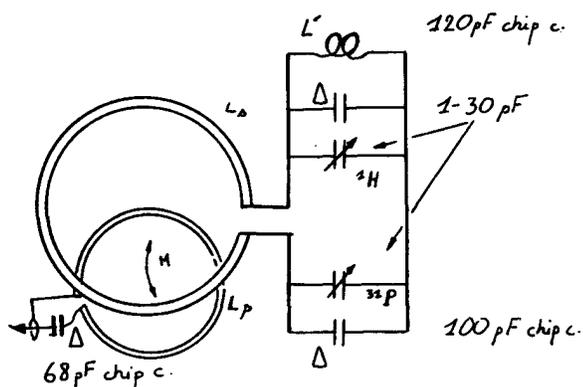
Figure 1. Electrical circuit of the two coil system (One side only).
