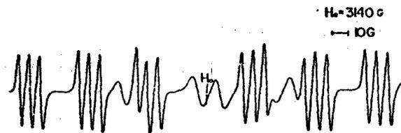
Fig.1 EPR spectrum of the radical ion at 77 K after irradiation at 77 K and annealing until 236 K
